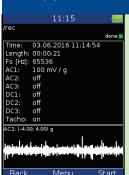
Recorder mode "records" the raw signal from the sensor (it means raw signal from the machine.) This allows you to make a post processing of the signal later on your PC.
